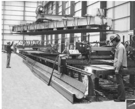
Multiple Selecto Magnets on a lift beam efficiently handle large steel sheets. In this installation, plates up to 10' x 50' x 4" (3 m x 15 m x 102 mm) are sorted and transported. The operator has precise remote control of every magnet so those not in use can be turned off, and single sheets can be dropped when desired from multiple-sheet lifts.
