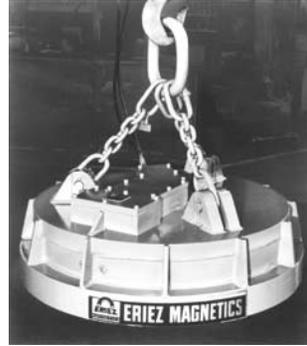
Eriez' Circular Lifting Magnets, with computer-designed magnetic circuitry, offer a high lift-to-weight capability in many applications: in steel mills, ball mills; for furnace charging and other materials-handling jobs.
