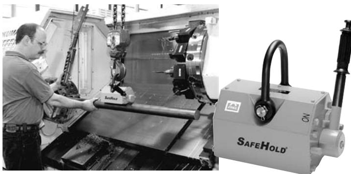
Lift, move or position round or flat materials with the same magnet. Specially designed poles on this new series of magnets allow the user to lift round materials up to 2,200 pounds. SafeHold® Lifting Magnets make quick work of difficult, time-consuming steel handling.
