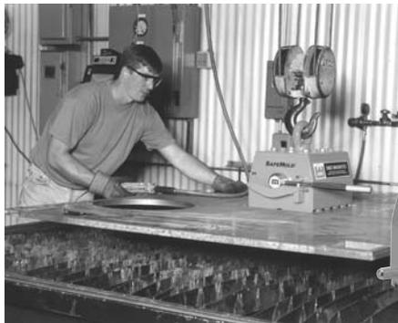
EPL Series SafeHold® Magnets are ideal for many machine-shop operations including the loading and unloading of this burn table.
