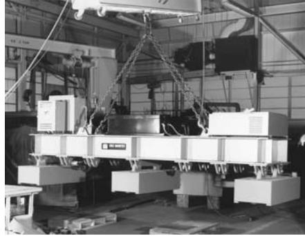
Powerful, computer-designed magnets up to 8' (2.4 m) long to lift, move and position heavy beams, channels, bars and flat steel plate
