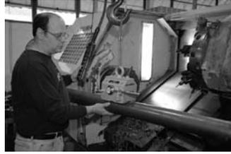
Eriez' XPL Series SafeHold makes easy work of this round bar stock. It handles flat sheet and plate steel with equal ease.
