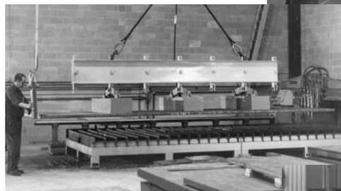
Heavy-Duty Rectangular Magnets provide maximum efficiency in multiple-plate handling applications like this.
